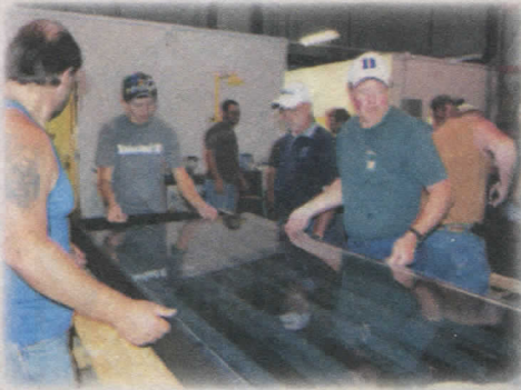
Sealing the box with glass reused from sliding doors will trap the heat inside this solar-powered water heating system.
